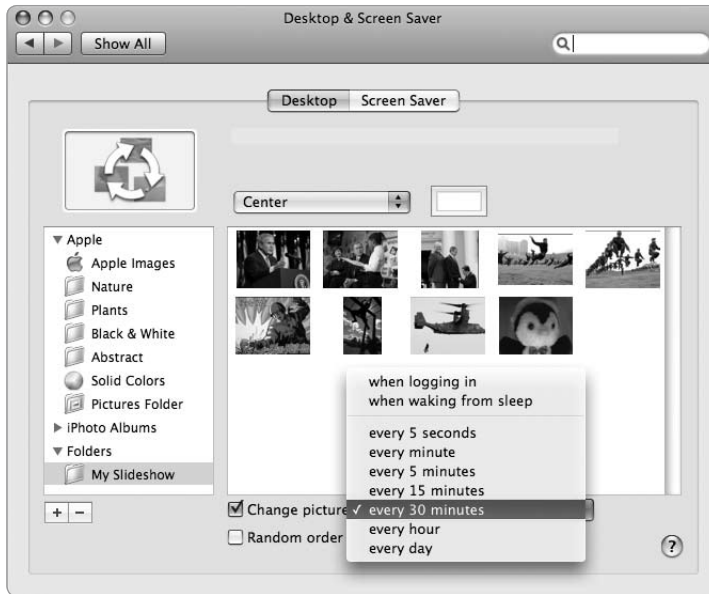
FIGURE 29-6: The Change picture pop-up menu lets you define how often a new picture appears.
